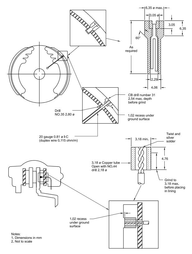
Figure 1 — Typical Plug Type of Thermocouple Installations
